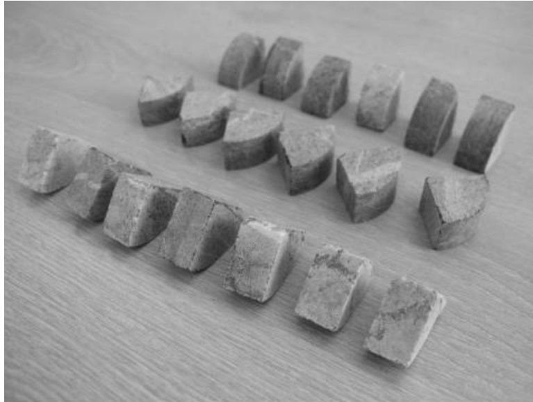
Figure 9 – Sample Pieces Cut from 50mm Quartered Core
