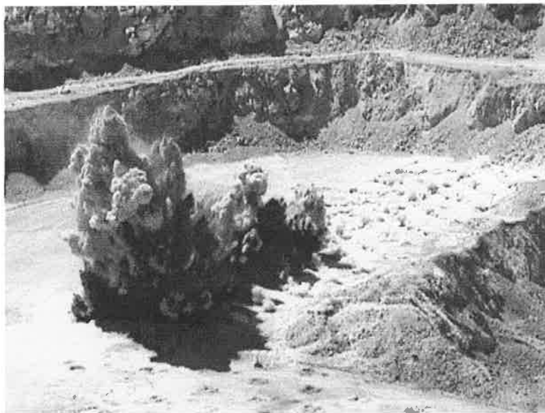
Figure 6 Cratering of Blasthole Collars
