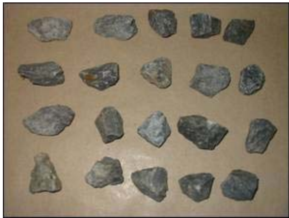
Figure 2 – Pieces Obtained by Crushing Drill Core
