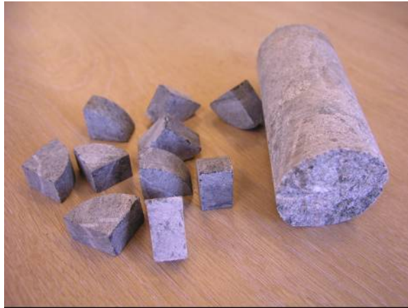
Figure 1 – Pieces Cut from a Drill Core Using a Diamond Saw
