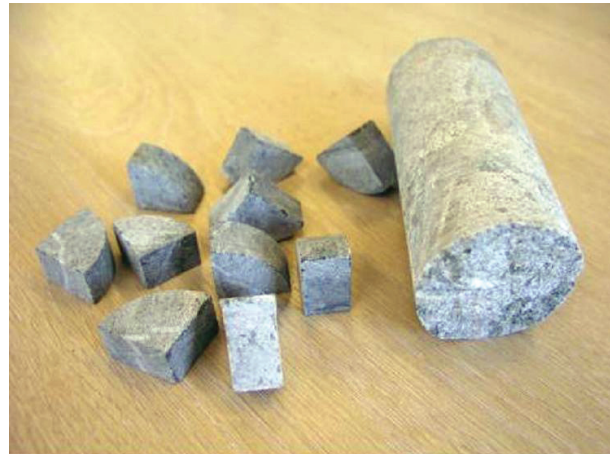
Figure A2. Particles Selected for SMC Testing from Cutting a Drill Core
