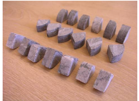
Figure 1 – Sample Pieces Cut from 50mm Quartered Core
