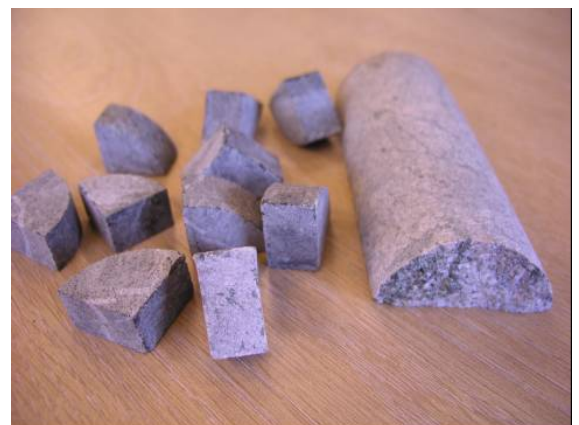
Figure 3 – Sample Pieces Cut from Half 50mm Core
