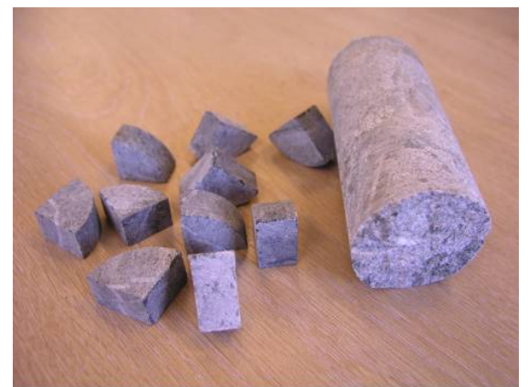
Figure 2 – Sample Pieces Cut from Whole 50mm Core
