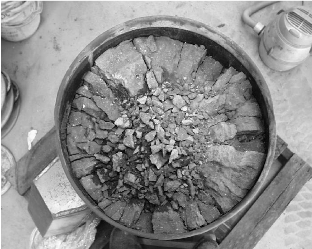
Figure 9 – Picture of Comminution Zones in Drum Blast
