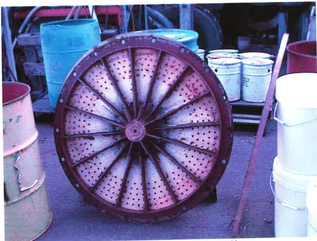
Figure 2 – Example of a Radial Pulp Lifter
