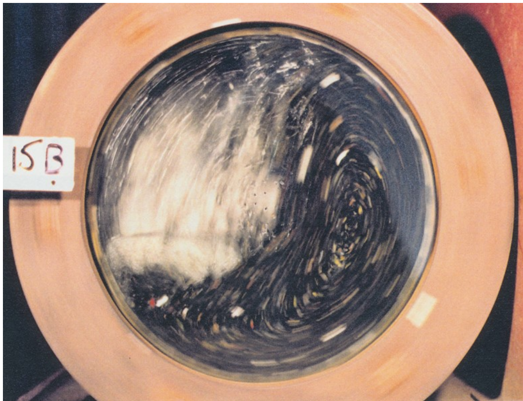
Figure 3.2a: Photograph of a 45% Mill Filling at 73% of Critical Speed
